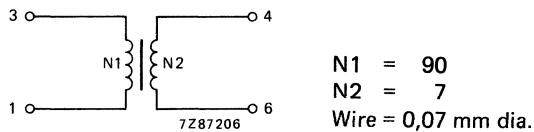
Fig. 12 Oscillator coil (L2). TOKO sample no. 7 BR-7 P.
